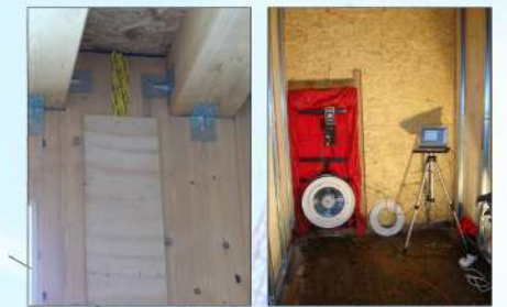
Nastrature/sigillature interne e Blower-Door-Test
